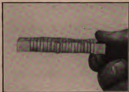
FIG. 255.—Twenty-two Gages Support Each Other.
